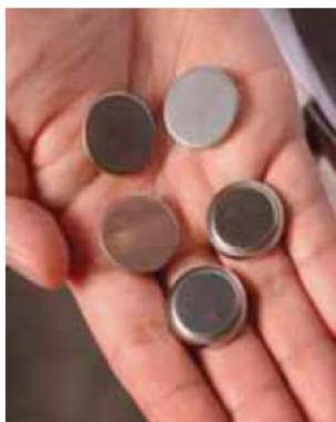
Fig. 2. Photograph of 2032 coin cells containing Si/C nanofiber anodes and/or LiFePO 4 /C nanofiber cathodes.
