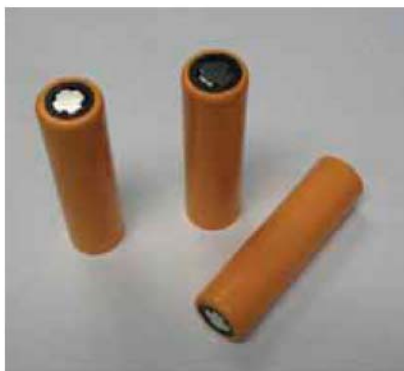
Fig. 8. Photograph of industry-standard 18650 cylinder cells containing Si/C nanofiber anodes.
